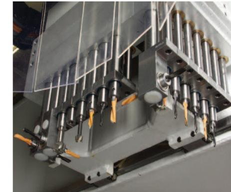
In addition to the basic equipment of one routing spindle, an optional tool interface HSK-F63 and a multi-spindle drilling box with 15 or 25 individually controllable spindles are available. The power consumption of a routing spindle with water-cooling is permanently controlled; this protects the spindle from damage.
