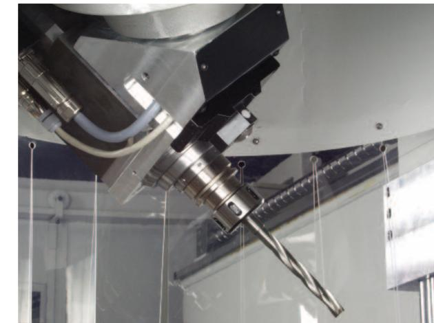
The ARTIS-X is equipped with a full 5-axis control – the Siemens 840Di sl. Digitally driven axes with absolute measuring systems, together with process optimised control functionality, guarantees the best machining results.
