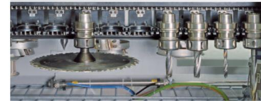
The aggregates move within the enclosed gantry – the tools making all the movements. The moveable automatic tool changing systems with up to 36 places (chain magazine) and a maximum outer diameter of 300mm, enabling the use of larger tools and standard additional heads.
